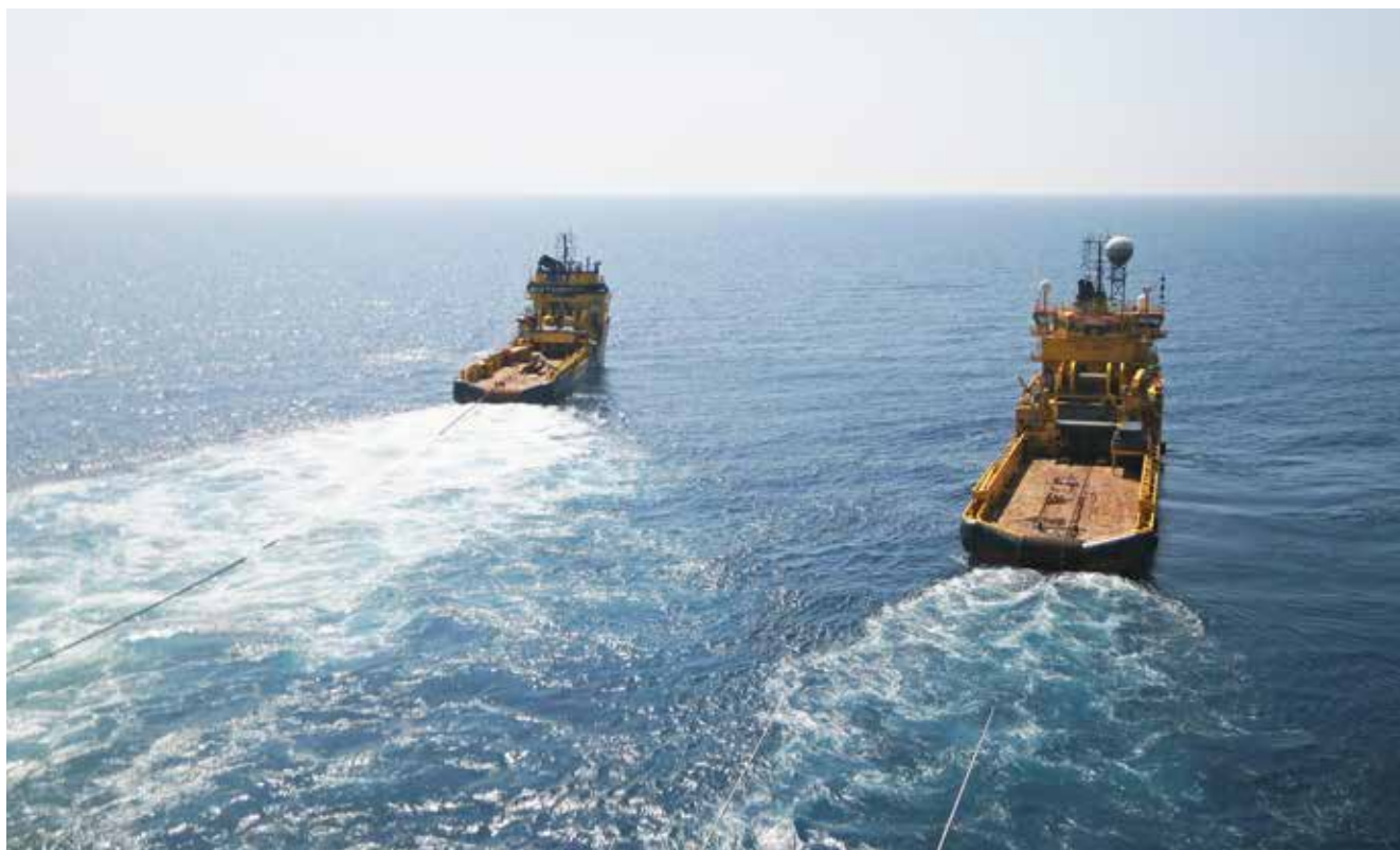
Odin Viking and Tor Viking running out two anchors for Stena Spey at Alma field in Central North Sea May 2014.
